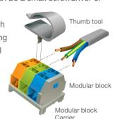
Once the cable is securely inserted remove your thumb tool or screwdriver from the modular block, the cable will now be connected, repeat until all cables have been inserted.
