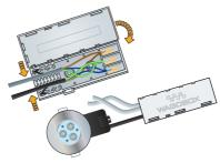
If required, the Wagobox 221-4 can be fitted to a surface using the Wagobox mounting button feature.
