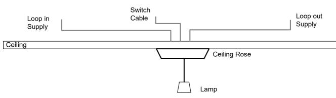
**NOTE:** This configuration is only applicable where the connected luminaire can be connected using a solid core cable and is a Class II accessory that does not require an earth connection
